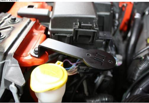
Use the M4x10 screws to attach JLT Separator to the JLT Bracket. Route long hose down and up along the wire harness. Plug on to the fitting on the supercharger and plug the short hose on to the fitting on the valve cover.
