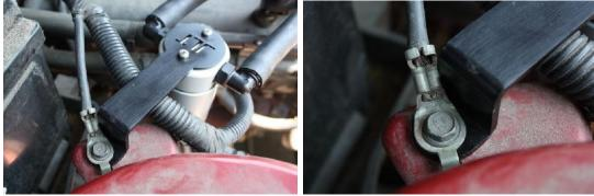
3) Use supplied screws to attach Separator to the bracket and hook up the hoses
