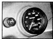
Slide speedometer into the mounting hole from the front side of the dashboard. Align mounting studs with mounting bracket behind meter. Attach with provided hardware.
