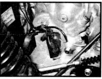
Trace harness to other bagged connection near vehicle transmission. See image at left. Remove bag and connect plug to supplied vehicle speed sensor.
