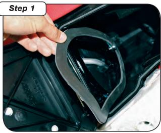
Remove seat/open airbox cover and remove foam air filter. Thoroughly clean sealing surface with parts cleaner and/or rubbing alcohol. Remove paper backing from foam gasket. Carefully adhere foam gasket to sealing surface of the air box. Press firmly into place.
