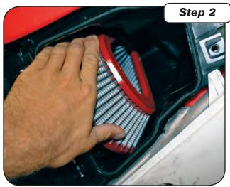
Place only the filter into the airbox and position around the mounting ring.
