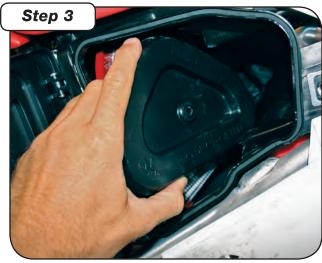
Hold the filter in place and position the plastic filter top over the filter. Insert the bolt and washer into the hole in the filter top and tighten until snug. Do not overtighten.
