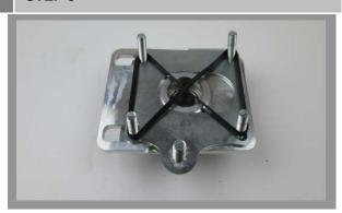
Place the Caster Plate on top of the bearing plate. Make sure that the raised lip around the bearing plate protrudes up through the center slot of the Caster Plate. NOTE!!! The use of a rubber band will help hold the stud plates in position while installing. Be sure the plates move from side to side smoothly.
