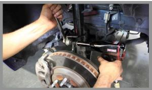
Remove the sway bar end link from the strut, then loosen but do not remove the strut mounting bolts.
