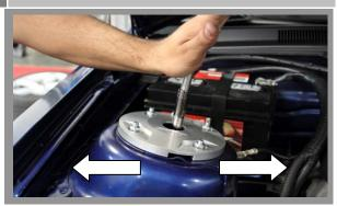
Center the strut shaft in the strut tower opening side to side. Once its center then tighten the 4 13mm nuts.
