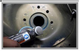
Check the bottom of the strut tower housing for any roughness. Use a Sander or sand paper to smooth out the Housing. NOTE!!! Must be smooth to allow the Camber/Caster Assembly to slide freely when adjusting.
