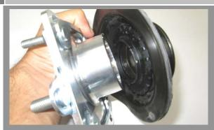
Install the Camber/Caster Assembly to the supplied Ford Strut Tower Pivot Assembly. NOTE!!! Use extreme caution, once the Camber/Caster Plate is installed to the Pivot Assembly it CAN NOT be removed. If removed it can cause serious damage to the top strut mount.
