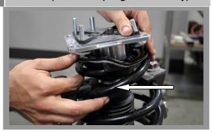
Place the Camber/Caster Assembly onto the Strut Assembly. NOTE!!! There is a supplied spacer for the 2005-2010 Mustang GT Models that needs to be placed onto the strut shaft before sliding the Camber/Caster Plate on.
