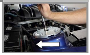
Loosen the 5 nuts on the Camber/Caster Plate assembly very slightly, until the plate can barely slide. Slide the entire assembly towards the rear of the vehicle and tighten the 17mm Nut.
