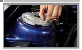
Re-install the strut assembly, place the cover over the strut tower where the studs protrude. don't fully tighten the top nuts. The factory strut tower brace can be used with this kit by placing the 2 ends above the decorative cover. NOTE!!!Remember to remove the rubber
