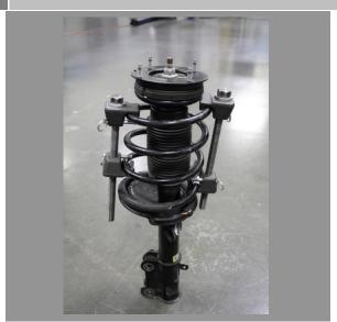
With a spring compressor, slowly depress the spring, then remove the upper strut retaining nut, then remove the upper strut mount assembly from the strut shaft. NOTE!!! Recommend the use of an impact gun.
