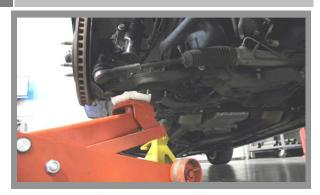
Support the lower control arm with a floor jack, remove the lower strut mounting bolts and lower the floor jack to remove the strut assembly.
