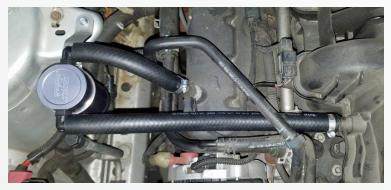
After assembling Oil Separator Kit as shown in pic install it on the vehicle with supplied hardware and clamping down hoses at valve cover/intake manifold connections and strut tower mount.
