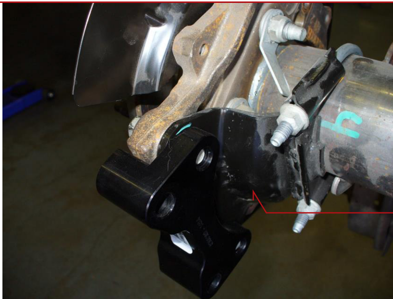
View of driver's side with intermediate bracket installed with anti-groan brace.
