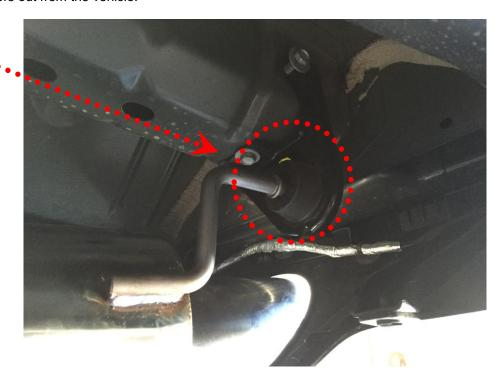
□ Slide the LTH<sup>™</sup> Axle-Back sections onto the factory mid-pipe where you made the cut previously. Be sure to slide a 2.50" exhaust clamp onto each pipe section before installing the LTH<sup>™</sup> Axle-Back sections.
