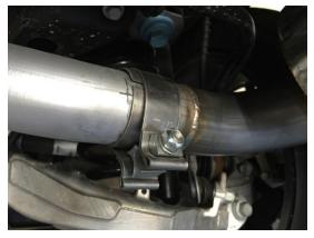
□ Slide each LTH™ Axle-Back section hanger into the factory rubber hanger by the cut-out in the rear bumper.
