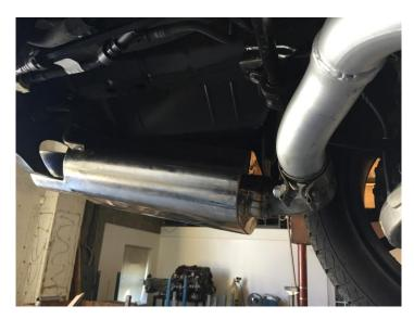
Adjust how much tube slides into or out of the factory pipe to adjust the position of the tip within the bumper cut-out. Once a desired fitment is achieved, tighten down the exhaust clamp. It may be easiest to have a helper position the exhaust, while you adjust for fitment at the tip to achieve an ideal position.
