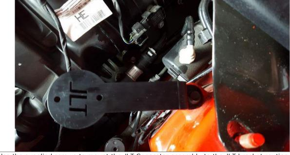
Use the supplied screws to mount the JLT Separator assembly to the JLT bracket routing the J hose(J Side of can)down toward the engine mount to connect to the PCV, and the T hose (T Side of can) under the intake for the fitting behind the throttle body
