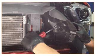
**33.** Push downward on the lower air diverter to release the six tree-clips that secure it. Once the air diverter is loose, push both radiator ducts inward, and slip the air diverter out to remove it from the vehicle. (6x tree-clips)
