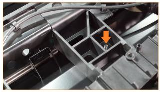
37. Install the two beveled spacers to the corners of the air diverter, and secure them with the two long bolts. When installing the beveled spacer, make sure that the beveled edge is on top. Loosely thread the nuts onto the bolts, and rotate each spacer until it is flush with both the radiator support and the air diverter. (2x beveled spacers, 2x 10mm long bolts, 2x 10mm Nylock nuts)
