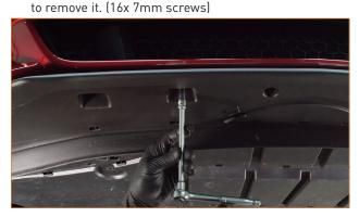
**04.** Remove the four screws that secure the rear splash panel to the vehicle. Then remove the splash panel from the vehicle. (4x 7mm screws)
