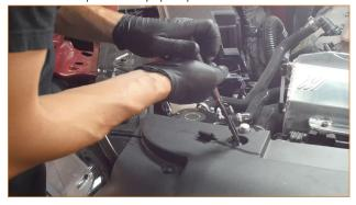
11. Remove the six screws that secure the top edge of the bumper. (6x 8mm screws)
