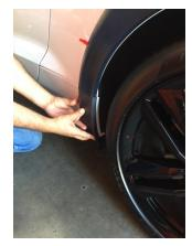
Step 10: Install small lower street flare by aligning top edge to fender line. Do not remove red backing from tape until fitment is confirmed.
