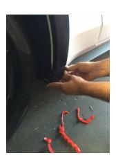
Step 6: Install small lower street flare by aligning top edge to fender line. Do not remove red backing from tape until fitment is confirmed.
