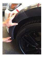
Step 5: Install bumper street flare by aligning front edge to bumper line. Do not remove red backing from tape until fitment is confirmed.
