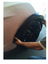
Step 8: Install large rear street flare by aligning front edge to lower fender line. Do not remove red backing from tape until fitment is confirmed.
