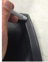
Step 2: Apply the provided 3M adhesive promoter onto the part and press the tape on.
