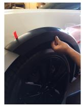
Step 4: Install large front street flare by aligning front edge to bumper line. Do not remove red backing from tape until fitment is confirmed.
