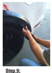
Install bumper street flare by aligning front edge to bumper line. Do not remove red backing from tape until fitment is confirmed.
