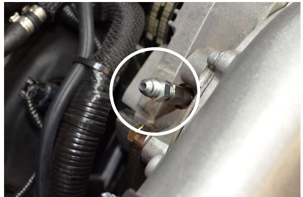
Fig. 11-b: -4AN Oil Feed Fitting Installed
