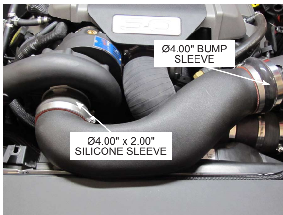
Fig. 8-b: Attach Air Inlet Duct To Air Box
