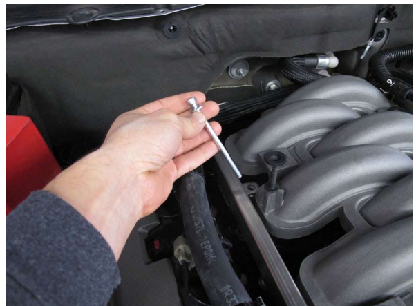
Fig. 6-f: Re-securing Fuel Rails
