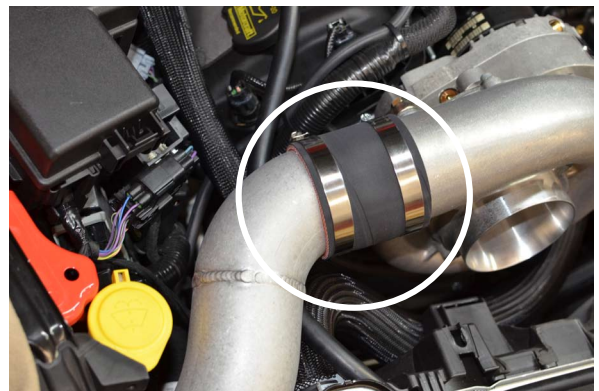
Fig. 5-f: Tube A Installation
