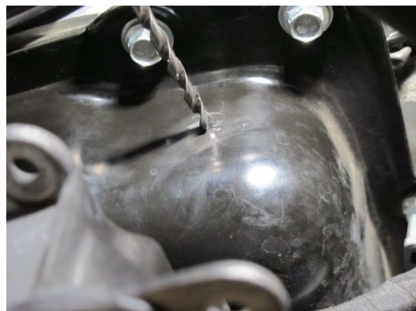
Fig. 12-c: Drill Pilot Hole
