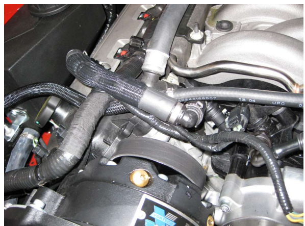
Fig. 4-c: Modified Passenger Side PCV Hose
