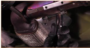
03. Remove the two bolts that secure the rear exhaust hangers to the rear subframe behind the differential. Lift the exhaust system slightly, and slide the hook on the front of the hanger out of the subframe. (2x 13mm bolts)
