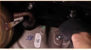
04. Separate the exhaust system from the flex section. Grasp the flex section and push the exhaust system straight back toward the rear of the vehicle. The stock exhaust system is heavy, so get a friend to help.
