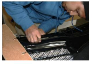
**Step 11:** Reinstall the trunk cover, if applicable, and finish the emergency trunk release hook and latch if these weren't completely finished.
