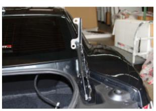
**Step 5:** You should perform a quick test fit of the carbon fiber trunk. The Anderson Composites trunk should already be open and inspected for shipping damage upon delivery from the trucking company. Remove the wooden legs from the trunk. Place the trunk where it will be easy to work with.
