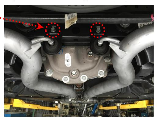
Finally, use a pair of exhaust hanger pliers to remove each of the rear tips from the exhaust hangers by the rear valence. You may want a second set of hands for this step. Once they are removed, you will want to pull the entire rear section of the exhaust from the resonator backwards and then drop everything down.
