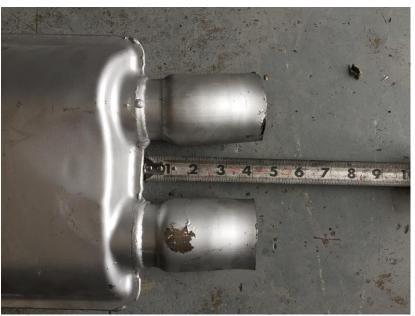
We can now begin the installation of the LTH™ resonator delete x-pipe. The x-pipe is not symmetrical and will need to be installed in a specific orientation to mate up properly with the factory pipe where you made your cut. The leg with the sharper bend near the outlets mates up with the passenger side piping, as shown.
