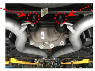
□ Finally, reinstall the rear mufflers into the exhaust hangers by the rear valence. Once everything has been fully supported, adjust the position of the tips in the rear valence if necessary, and then fully tighten the 2.50" exhaust band clamps and the factory clamps at the front.
