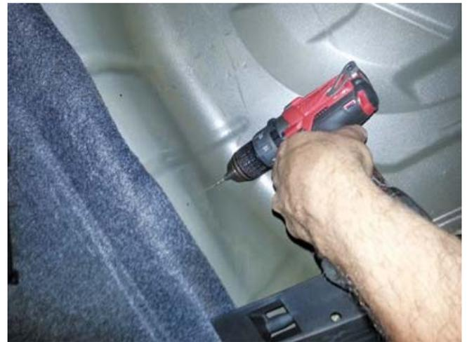
3. Using the #8 self-tapping screws, attach the fuel pump voltage regulator to the wheel well.
