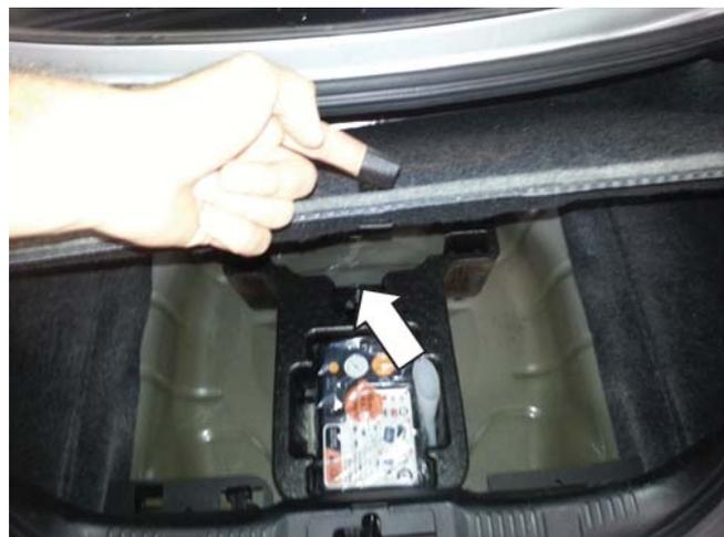
5. Remove the plastic taillight closeout panel (there are four [4] end caps holding the closeout panel on).
