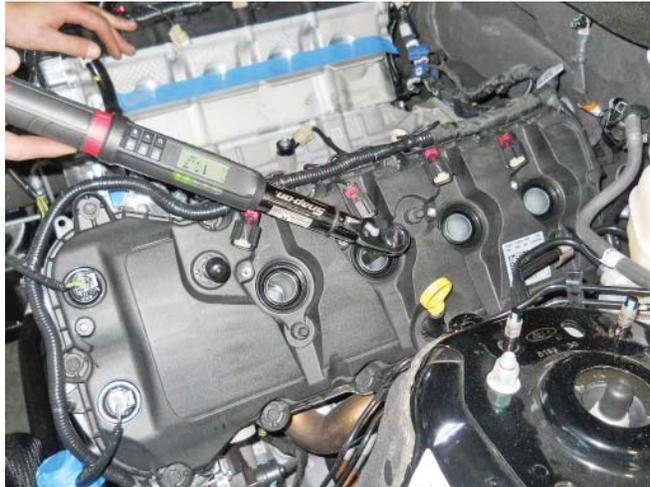
17. Apply a small amount of dielectric grease and reinstall the ignition coils, torquing the bolts to 6 Nm.
