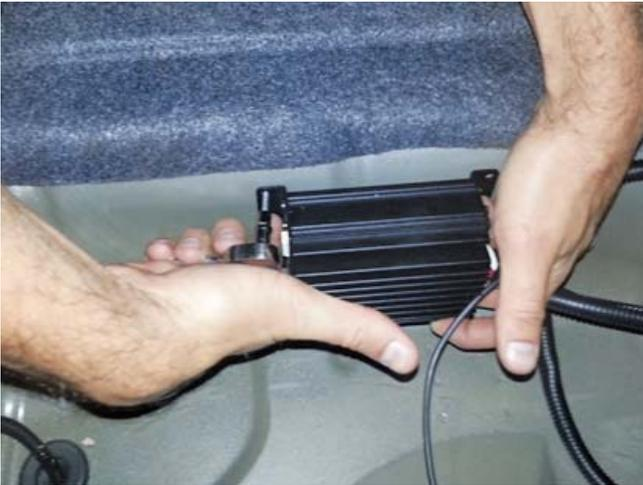
4. Attach the ground strap to the chassis ground of the driver side of the trunk.
