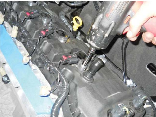
13. Remove the ignition coils and number them so they can be reinstalled in the position from which they were removed.
