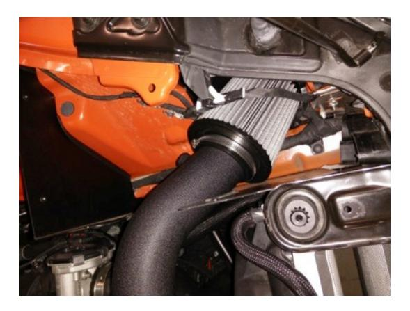
8. Take the Intake Engine Mount Bracket and the 2 flange head M12 x 30 bolts with the 2 corresponding 12mm flat washers and lock washers and loosely fasten the bracket to the front engine mount. Use a 17mm socket to tighten.
