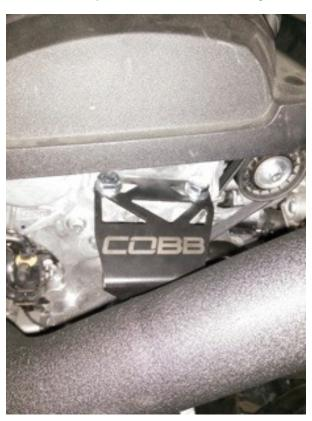
9. Now you can move the Intake Pipe to where you are able to loosely fasten the pipe to the bracket using an M8 x 12 Flange Head Bolt
