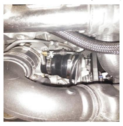
3. Install the COBB 3" Intake Pipe into the turbo silicone. Make sure the side that goes into the turbo silicon has the bungs to reattach the BPV and PCV. Apply some silicone spray if needed. Loosely install the 048 worm clamp to hold the intake pipe to the silicone reducer coupler.
