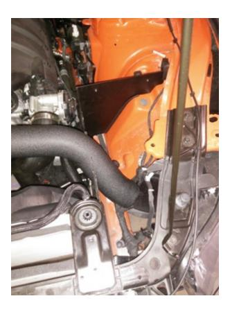
6. Using the M6 flange head bolt and the 6mm nylon washer, bolt down your new airbox using a 10mm socket in the same location using the mounting slot on the COBB Airbox. Tighten both bolts used to install the airbox.
