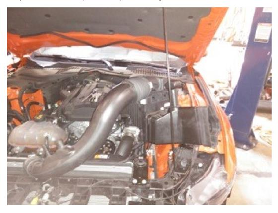
5. Remove remaining stock silicone hoses and the grommet used to hold the stock intake in place. If needed you can take the airbox out first and then the intake tubing if you are unable to remove it all at once easily.
