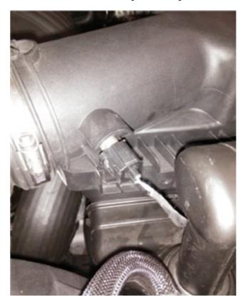
3. Remove the bolt that is holding the back of the airbox in place with a 10mm socket.
