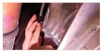
**05.** Remove the two nuts holding the bracket to the downpipe, and then remove the plate under the bracket. (2x 13mm nuts, 1x plate)
