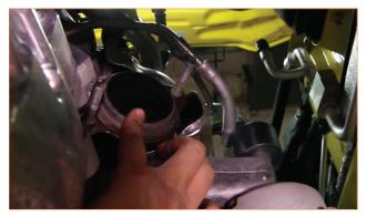
**11.** Remove the O2 sensors from the stock downpipe using a 22mm wrench. Note the position of each sensor as they are different.
