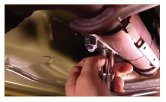
**08.** Lubricate the rubber grommet, and push the hanger on the downpipe out of the grommet.
