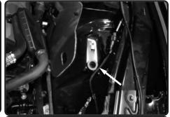
11. Install the larger grommet from figure 8 and install it into the original hole location on the fender well
