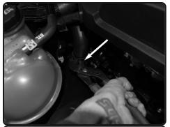
**5.** Use a channel lock wrench to loosen the tension clamp on the diverter valve return line to the factory air duct.
