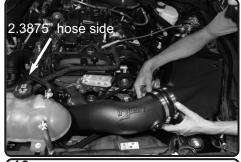
**19.** Place the intake tube into position. Slide the 2.3875" coupler onto the turocharger and then slide the 4.5" hump hose over the plenum. Adjust the intake for best fitment and then secure the clamps
