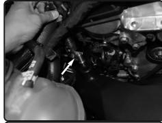
**20.** Connect the crank case fitting onto the Injen machined fitting on the intake tube. Make sure it clicks into place.
