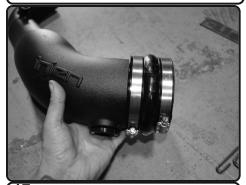
**17.** Place the 4.50" hump hose and 2 #72 clamps onto the larger end of the Injen intake tube.
