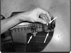
**8.** Remove the two grommets and spacer washer from the OE air box assembly
