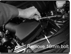
**2.** Remove the 10mm bolt from the side of the stock OE air box.
