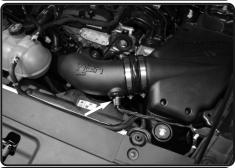
**22.** Screw in the Air temp sensor into the machined AIT sensor adapter.
