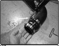
**18.** Place the 2.3875"-3.0" step hose and #48 and #36 clamps onto the smaller end of the Injen intake tube and only secure the clamp on the 3.0" side for now.
