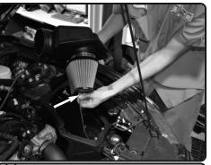
**14.** Connect the 3mm vacuum line from the filter minder to the barbed fitting on top of the filter.
