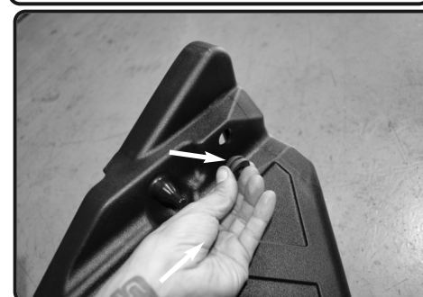
10. Install the smaller grommet and spacer washer from figure 8 into the 1/2" hole on the Injen lower air box assembly.
