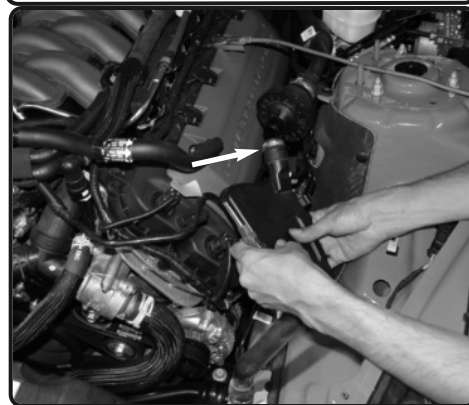
6. Disconnect the sound tube resonator box.
