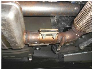
4) Using a 15mm wrench, loosen the two bolts at the clamp connection in the center of the vehicle. Use a small screwdriver to lift the clip and with the help of an assistant, carefully lower the stands at the rear of the resonator and slide the system toward the rear and off of the front pipe. Lower the resonator from the vehicle. The clamp should remain on the factory front pipe as it will be re-used with the new Flowmaster system.
