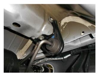
3) Using a 13mm wrench, loosen the two hangers just behind the rear differential from the cross member and the two hanger mounts at the rear of the vehicle from the frame. Slide the muffler assemblies toward the rear of the vehicle to disengage them from the factory system. Leave them hanging in place for re-assembly onto the Flowmaster Y-pipe assembly.
