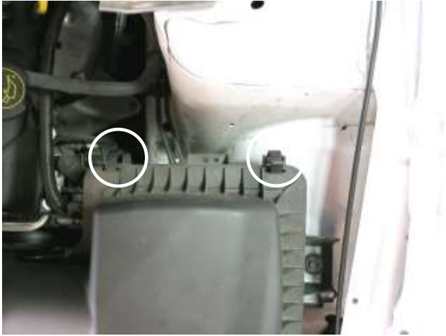
b. Reinstall the upper air box. Reattach the clips that were removed in step 2d.
