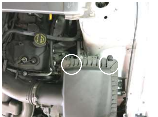
d. Unlatch the two clips securing the upper air box to the lower air box.
