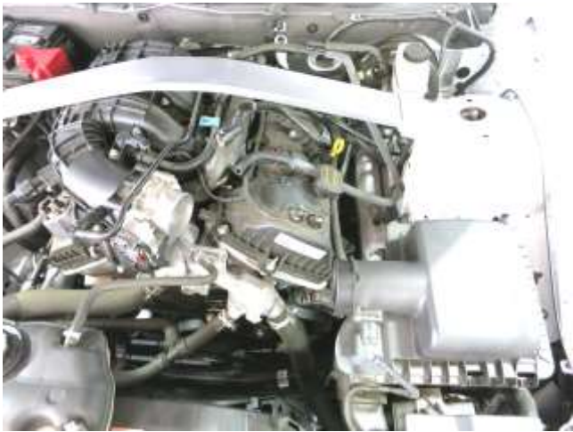
f. Remove the stock intake hose from the vehicle. Note: Do not discard any of your stock equipment.
