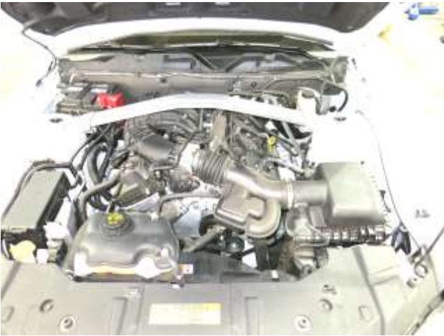
h. STOCK INTAKE INSTALLED
