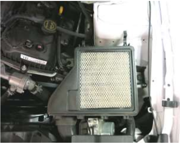
e. Remove the stock air filter from the lower air box.
