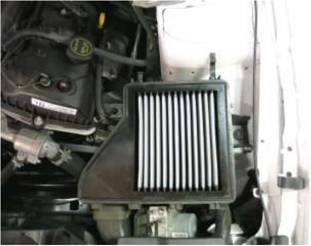
a. Install the AEM filter into the lower air box.
