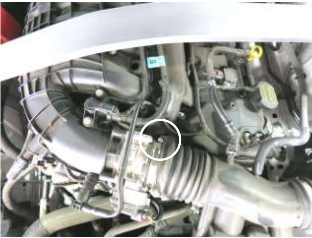
a. Loosen the hose clamp at the throttle body.
