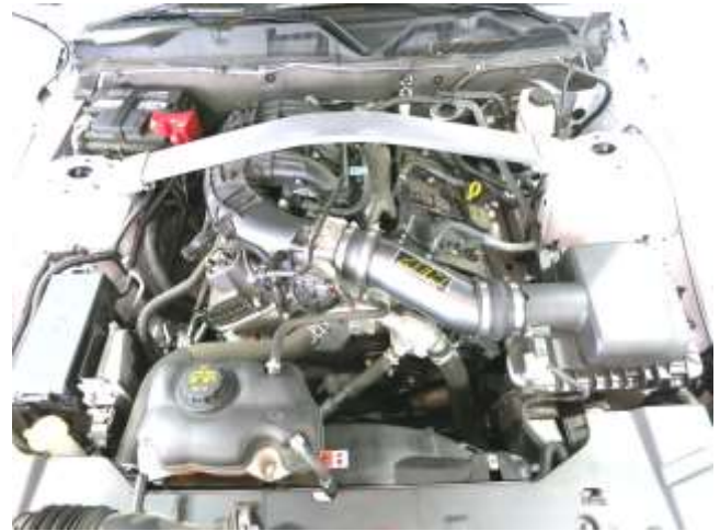
i. AEM INTAKE INSTALLED
