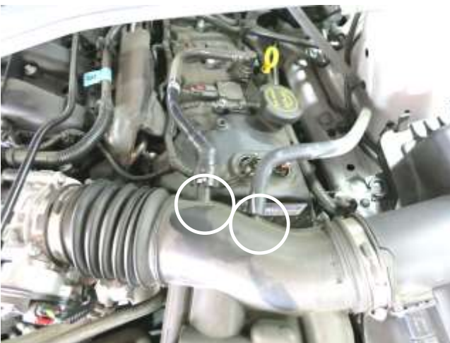
c. Release the pressure on the gray tab and pull the two vent lines from the stock intake tube. Note: Only automatic transmission models are equipped with an EVAP vent line.
