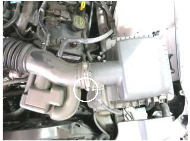
b. Loosen the hose clamp at the air box outlet.
