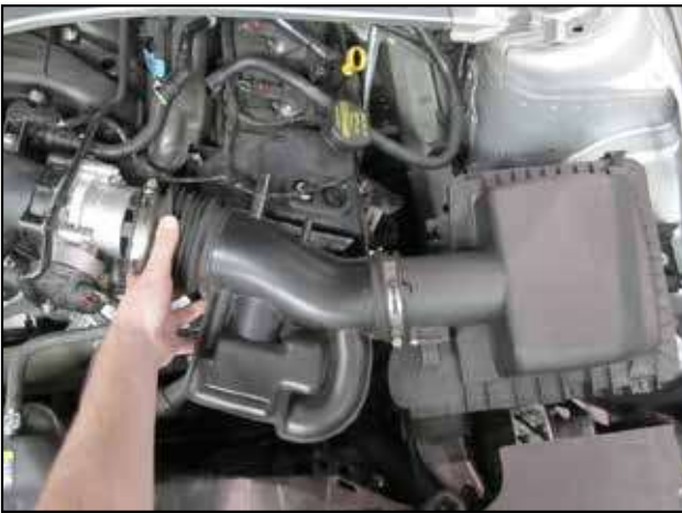
g. Remove the OEM inlet tube off of the throttle body.
