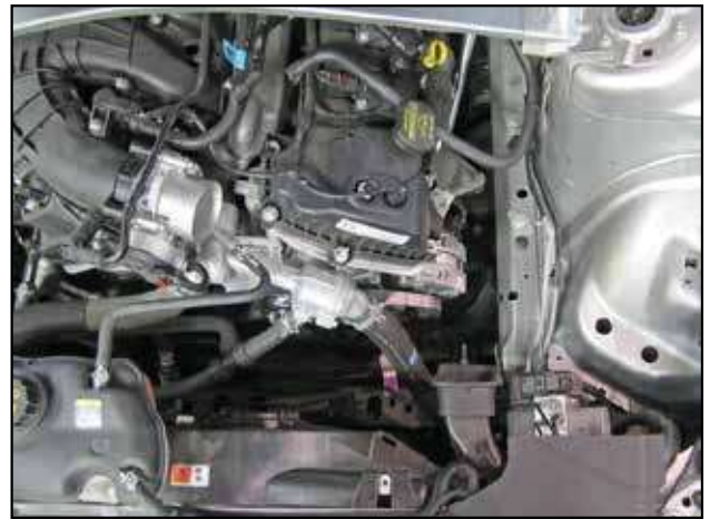
h. Lift up and remove the OEM airbox and intake tube from the vehicle.
