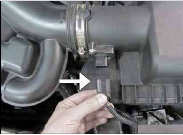
e. Unplug the MAF sensor connector.
