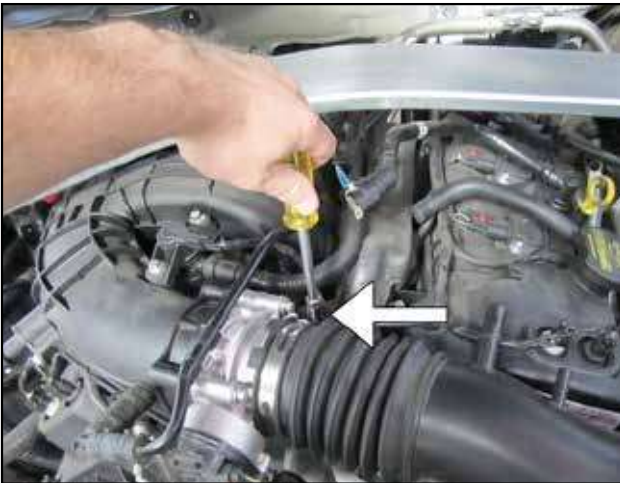
c. Loosen the hose clamp at the throttle body.
