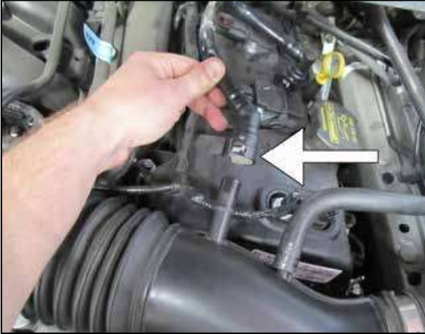
a. Disconnect the crankcase vent line.
