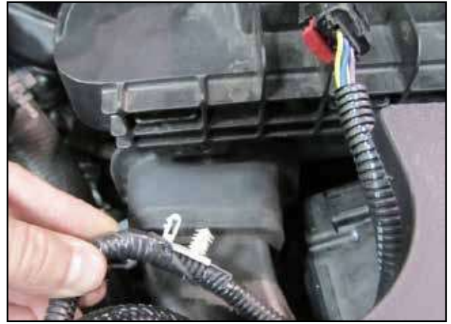
f. Unclip the MAF sensor wire harness from the airbox.
