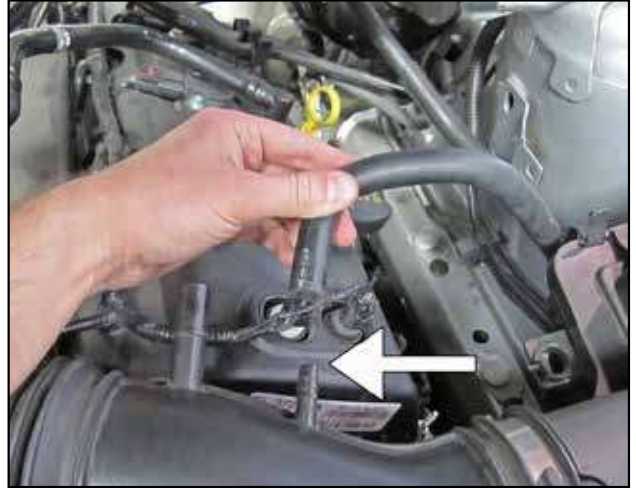
b. Disconnect the brake booster vacuum line.
