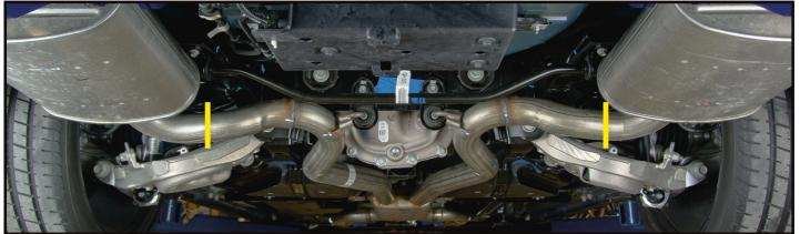
Cut the factory system close to the bend that leads to the muffler. This will give you the maximum amount of material for adjustments.
