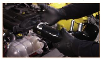
**11.** Reconnect the quick-disconnect fitting. You should hear the plastic tabs snap into place.
