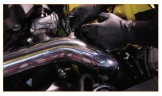
**32.** Attach the large rubber strip to the airbox lid. One end must sit flush, while the other end should extend about 3/4" for clearance.
