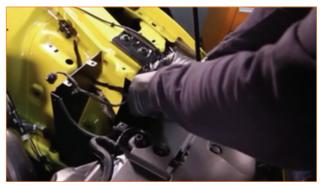
**25.** Insert the intake pipe and air filter into the engine bay. If the filter fitment is tight, turn the assembly slightly during install.
