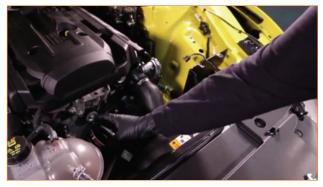
**24.** Remove the tree clip holding the wire harness to the body of your Mustang.
