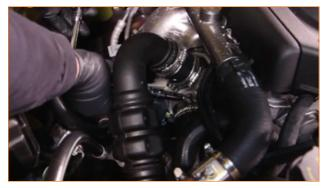
**29.** Fully tighten the 10mm nut that holds the rubber bushing to the body of your Mustang.
