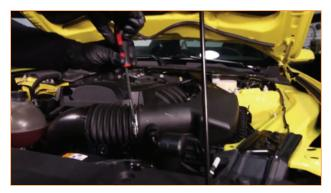
$\ensuremath{\textbf{2.}}$  Disconnect the plug from the intake air temperature (IAT) sensor.
