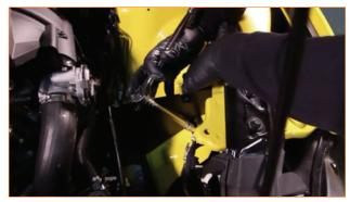
**18.** Install the two tree clips on the bottom, starting with the rearward tree clip.
