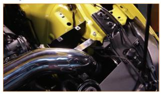
**27.** Position the intake pipe into the inlet hose. The hose should have some room to move. Fully tighten the large worm-gear clamp.
