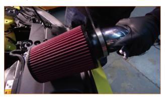
**21.** Attach the upper rubber bushing to the intake pipe. The unused threads must be facing upward. (10mm ratchet wrench)
