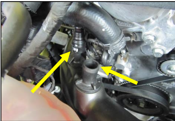
6. Disconnect the PCV and turbo bypass lines from the intake tube and remove the tube from the vehicle.
