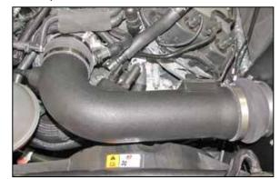
24. Install the K&N® intake tube into the hose at the filter adapter and then into the hose at the throttle body, adjust the tube for best fit and then secure with the provided hose clamps.
