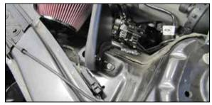
16. Secure the heat shield to the air filter housing mounting location using the provided hardware.
