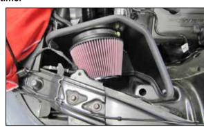
15. Install the K&N $^{\circ}$  air filter onto the adapter and secure with the provided hose clamp.
