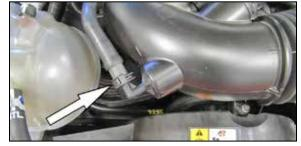
3. Depress the locking tab and then disconnect the idle bypass hose from the intake tube.
