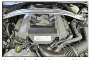
2. Lift up the decorative engine cover to dislodge it from the mounting studs and then remove the engine cover from the vehicle.
