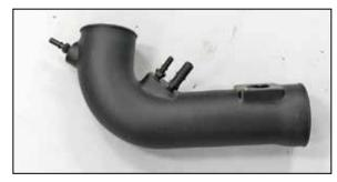
19. Install the quick disconnect fittings into the K&N® intake tube as shown.
