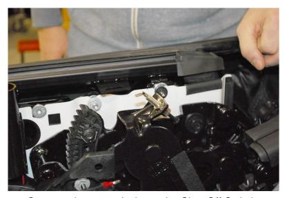
Connect the ground wire to the Shut Off Switch.
