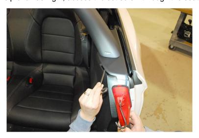
Tighten the set screw with a "T" handle ¼" Allen wrench (or similar). Apply slight downward pressure on the Lightbar to ensure a nice fitment to the trim panel, and tighten the set screw. Repeat on opposite side.
