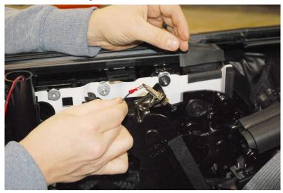
Drill (2) 3/16" holes in the speaker housing to and secure ground wire with zip ties as shown below.
