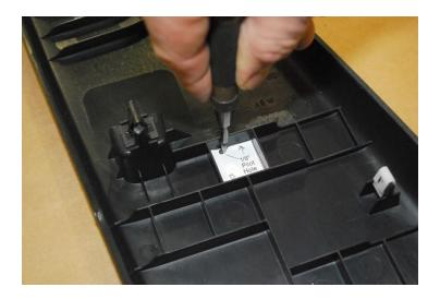
9. Drill panels with 1/8" pilot drill.
