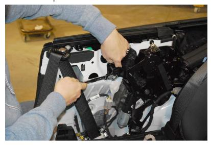
17. Install passenger side bracket. (Brackets are labeled.) Reinstall the 10mm window molding bolt, hand tighten at this time.
