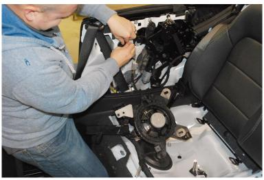
14. Remove rubber grommet. Set aside to be reinstalled later.
