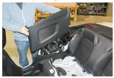
13. Remove speaker assembly attachment hardware. (3) 10mm nuts, and (1) 7mm hex head screw. Also need to remove electrical component from "B" pillar. (1) 10mm Stud, and (1) 7mm hex head screw.
