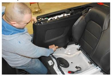
**HINT:** It's very helpful to release the plastic retainers that secure the panel to the speaker housing with a pair of needle nose pliers.
