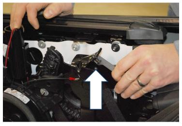
Using the supplied 5/16"-18 thread cutting bolt (1/2" head), re-thread the bump stop hole. Remove bolt and discard, it is only used to create the new threads.
