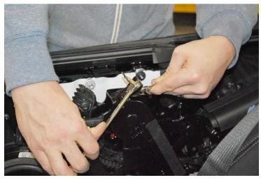
With a pair of pliers, bend the connector tab 90 degrees. As shown.
