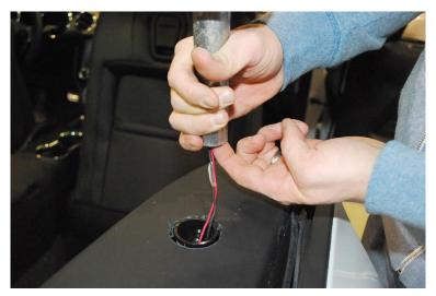
With the help of a flashlight, access the set screw through the seat belt slot.
