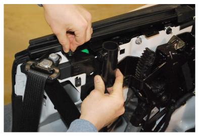
Reinstall the 15mm convertible top bolt, hand tighten at this time.
