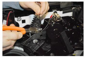
Depress the switch a couple times, paying attention to the travel of the switch. Make sure there is adequate length of wire, and not excessive length.
