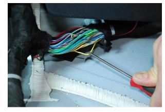
Connect the provided **RED T-Tap** to the **yellow/silver stripe** wire. Simply place the wire in the center of the metal tab of T-tap, fold the T-tap, and squeeze the T-tap with a pair of pliers. Rotate the T-tap a couple of times after it's been closed to ensure a good connection. Now, plug in the **SPADE CONNECTOR** from the Lightbar harness. **HINT:** Make sure the spade is in the center of plastic isolator.
