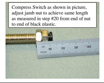
21. Install the plunger switch. Using your dimension from step #20, set the jamb nut. <a href="HINT: Adjusting the jamb nut like the previous picture should get you very close, adjust if needed.">HINT: Adjusting the jamb nut like the previous picture should get you very close, adjust if needed. Thread the switch into the bump stop hole so that the connector is facing up and toward the front of the car.
