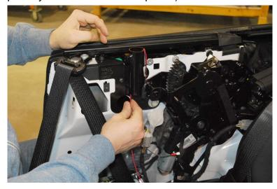
Route the positive wire (red) as shown, and use a provided zip tie to secure the harness to the existing wiring. **IMPORTANT:** Make sure to safely route wiring away from moving parts (seat belt retractor and convertible top mechanism).
