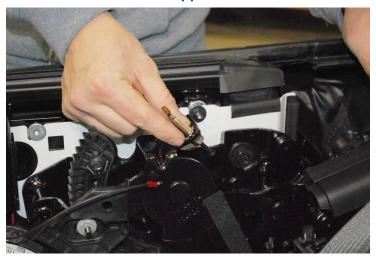
Install the provided nut with a pair of 12mm wrenches. WARNING: Do not exceed 60 IN-LB.
