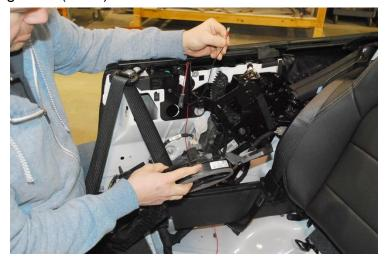
20. <u>READ this step completely before proceeding</u>. Measure the distance of the convertible top bump stop from the base of the bracket to head of the bump stop and record the measurement. Remove bump stop using a T-25 Torx bit, or an 11mm wrench.
