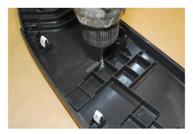
10. Flip panels over a drill 2" holes with hole saw, and set panels aside for later reinstallation.
