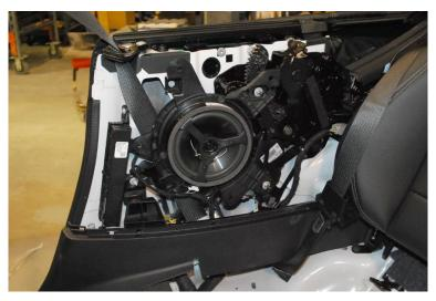
No need to disconnect the wiring, allow speaker to hang as shown in picture below. Place a cloth or rag between the panel and speaker bracket to avoid scratches on the quarter trim panel.
