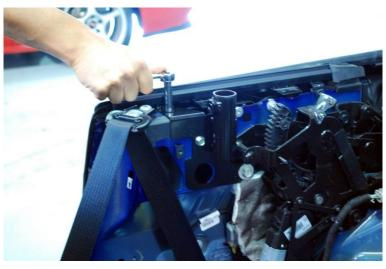
Install rubber grommet (removed in step # 14) into bracket as shown.
