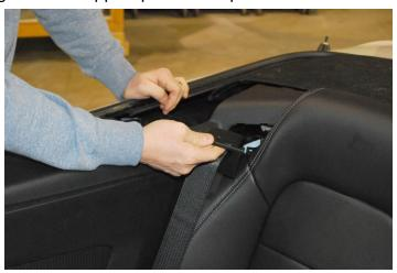
4. Dislodge the upper trim panels, but do not remove yet. Pull up evenly on panel to release the plastic retainers. **WARNING:** Do not pull too hard on the front of the panel at the seat belt area, as you may risk stressing the plastic causing permanent damage to the part.
