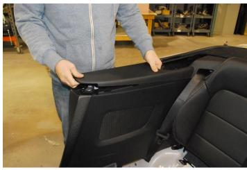
5. Disconnect electrical connector located behind the seat belt guide and remove upper quarter trim panel. **Note: Connector not present on all vehicles.**
