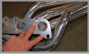
There are 2 thread pitches supplied. Because the manufacturer changed the thread pitch used after 2011 you will have to compare the supplied bolt to the factory stud to confirm which thread pitch to use.
