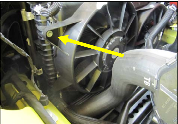
15. Remove the drivers side fan shroud bolt and set it aside.
