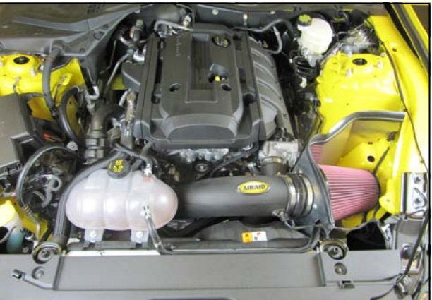
24. Double check your work. Make sure all clamps, hoses, bolts, and screws are tight. Double check the hood clearance. Reconnect the negative battery cable.
