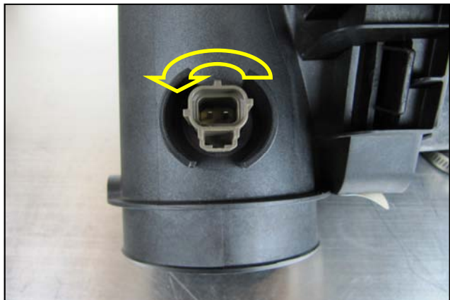
9. Tilt the air temp sensor rearward so the locking tab clears the ramp and rotate it counterclockwise 1/4 turn to release it.
