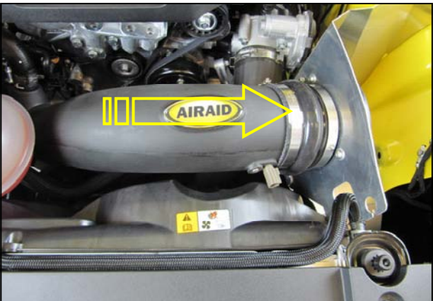
21. Slide the Airaid Intake Tube into the Hump Hose and tighten all four Hose Clamps. Apply the Airaid Bubble Decal onto the Intake Tube as shown.
