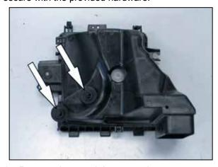
15. Remove the two air box mounting grommets from the factory air box.
