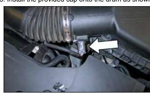
6. Disconnect the mass air sensor electrical connection.
