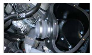
18. Install the provided silicone hose (08699) onto the filter adapter and secure with the provided hose clamp.
