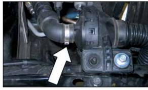
3. Cut the clamp that secures the engine pulse hose to the drum and disconnect the hose from the drum.
