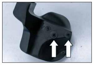
16. Install the air box mounting grommets onto the two mounting studs installed onto the K&N<sup>®</sup> air box.
