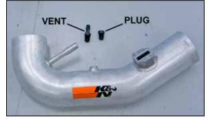
20. On vehicles that have an EVAP vent line attached to the intake tube, install the 3/8" vent fitting into the K&N® intake tube. On vehicles that do not have the EVAP vent line attached to the intake tube, install the npt plug into the intake tube. NOTE: Plastic NPT fittings are easy to cross thread. Install the vent fitting "hand" tight, then turn it two complete turns with a wrench.
