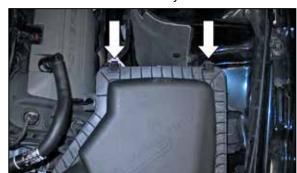
9. Release the two upper air box retaining clips.
