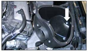
17. Set the K&N<sup>®</sup> air box into the vehicle so that the mounting studs slide into the mounting holes, then secure with the provided hardware.
