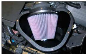
26. Attach the K&N® air filter onto the filter adapter and secure with the provided hose clamp.
