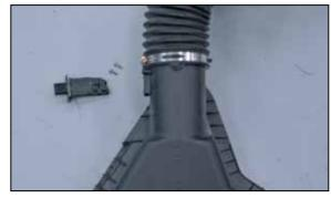
21. Remove the two bolts securing the mass air sensor into the factory intake tube and then remove the mass air sensor from the intake tube.
