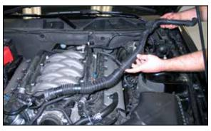
4. Release the clamp that secures engine pulse hose to the intake tube, then remove the engine pulse hose from the vehicle.
