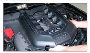
2. Lift up the engine cover and remove it from the vehicle.
