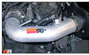
23. Install the K&N® intake tube into the silicone hose at the air box and then into the silicone hose at the throttle body; secure with the provided hose clamps.
