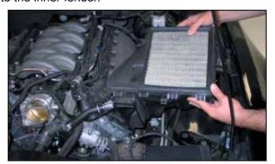
12. Remove the lower air box from the vehicle.
