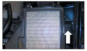
11. Remove the bolt that secures the lower air box to the inner fender.
