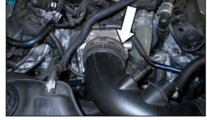
8. Loosen the hose clamp that secures the factory intake tube to the throttle body.
