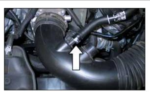
7. Disconnect the crank case vent hose from the factory intake tube.
