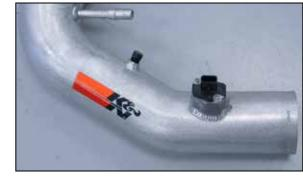
22. Install the mass air sensor into the K&N® intake tube and secure with the provided hardware.
