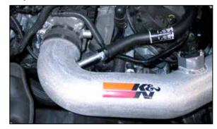
24. Connect the crank case vent hose to the fitting on the  $K\&N^{\scriptsize @}$  intake tube.
