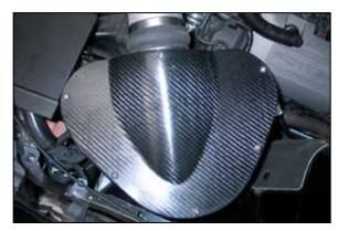
27. Install the  $K\&N^{\otimes}$  air box lid and secure with the provided hardware.
