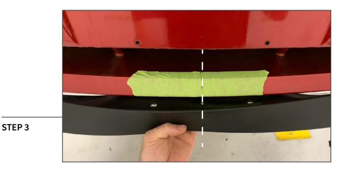
Measure to find the center point of the bumper. Using masking tape and a marker, mark the center of the bumper. Align the center hole of the chin spoiler with the center of the bumper.
