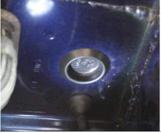
2013-14 GT has an open hood vent that can bring water into the filter area. If this is a concern to you, we have included a plug to keep the water away from your filter and still allow engine heat to escape.
