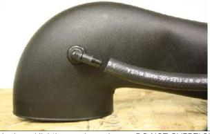
Attach JLT intake kit on to throttle body and lightly snug hose clamps. DO NOT OVERTIGHTEN CLAMPS!!
