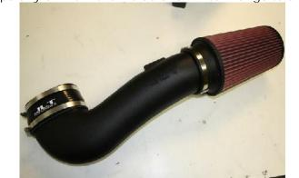
Install MAF sensor in the JLT MAF housing using supplied Phillips head screws and MAF gasket. Screws just need to be snug.
