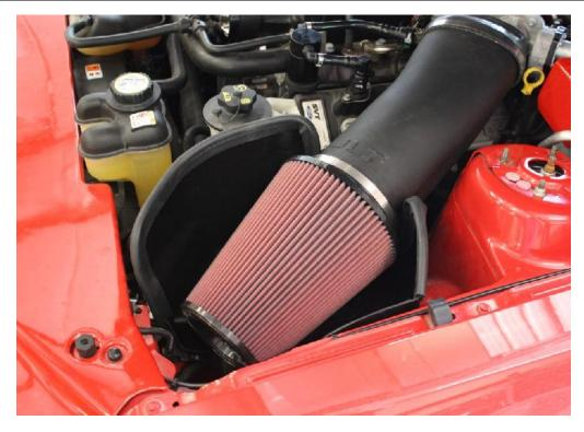
This kit includes an S&B Powerstack pre-oiled reusable air filter. The frequency you should clean your filter will depend on your driving conditions. It is recommended to check your filter at every oil change or 3,000 miles. If there is a build up of dirt as thick as the wire mesh, then it's time to clean your filter. As dirt builds up on your filter, the restriction of the airflow also increases. More frequent cleanings will improve your fuel economy and your vehicle's performance.
