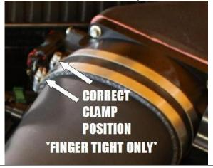
Plug in the PCV and MAF connections. Adjust tube in and out of throttle body coupler for best fit and DO NOT over tighten the clamps, they only need to be finger tight.
