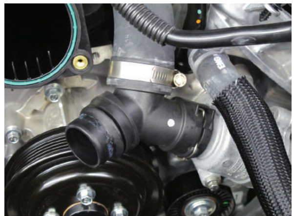
Fig. 2C: #28 Hose Clamp Orientation
