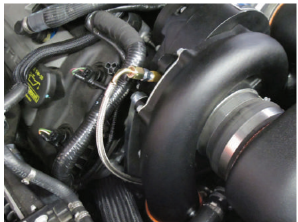
Fig. 13C: 90° Oil Feed Hose Installed
