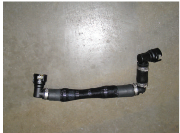
Fig. 5D-3: Modified Passenger Side PCV Hose
