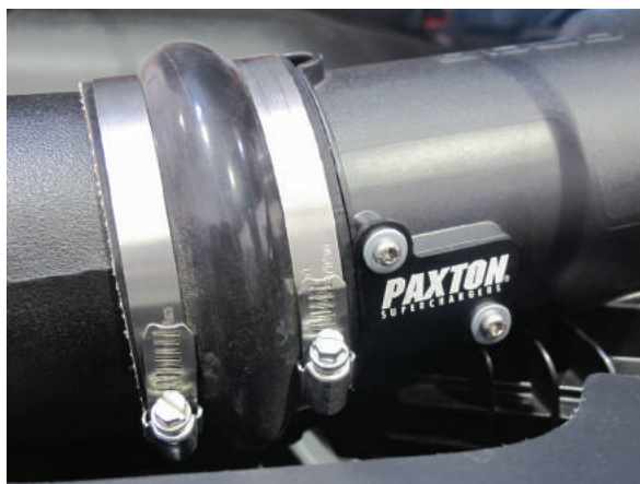
Fig. 11I: Air Inlet to Airbox Connection; MAF Port Cover
