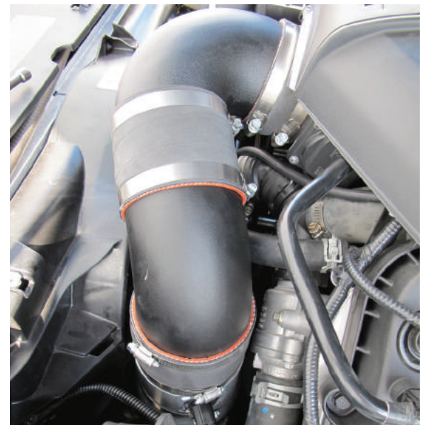
Fig. 7C-7: Cast Elbows, Final Position
