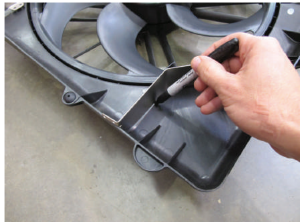
Fig. 3AD: Marking Air Dam Cut Lines
