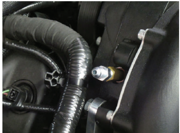
Fig. 13B: -4AN Oil Feed Fitting Installed
