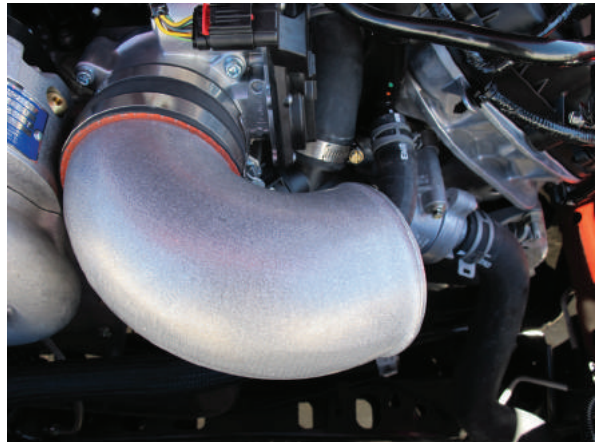
Fig. 7C-6: \text{\O}3.5 " x 120^\circ Cast Aluminum Elbow
