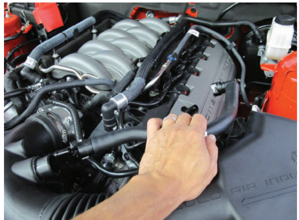
Fig. 1S: PCV Hoses
