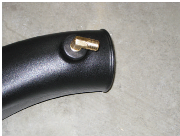
Fig. 11A: Air Inlet 3/8 NPT 90° Hose Barb Fitting
