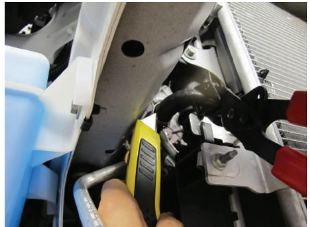
Fig. 2G: Clamping and Cutting A/T Hoses
