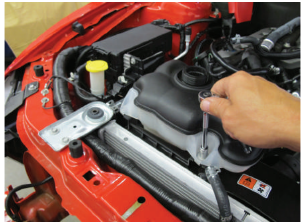
Fig. 1Z: Coolant Reservoir
