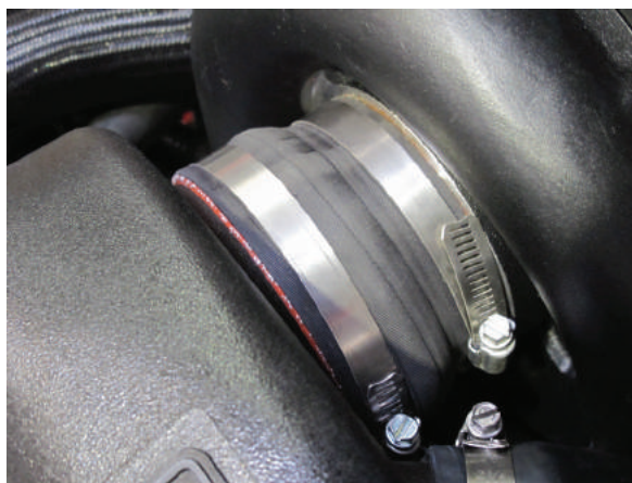
Fig. 11B: Air Inlet to Supercharger Connection
