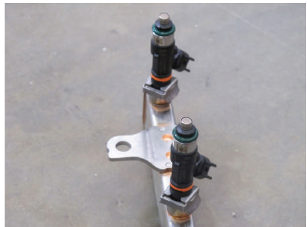
Fig. 9K: Fuel Rail / Injector Assembly Detail
