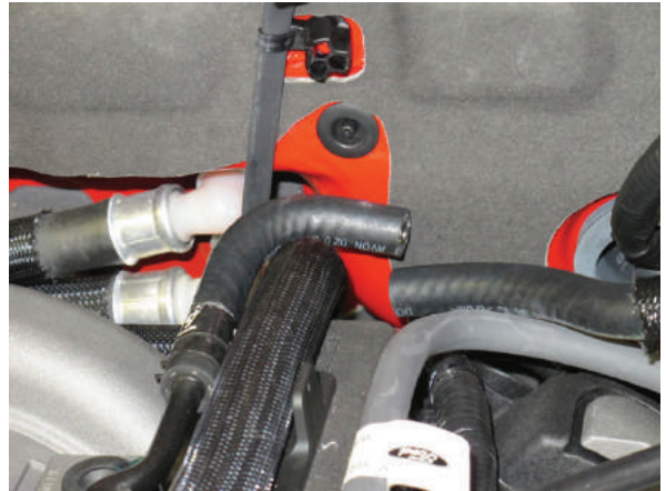
Fig. 8A-1: Vacuum Hose Cut
