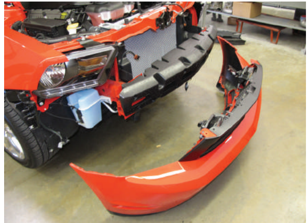
Fig. 1J: Front Fascia Removal
