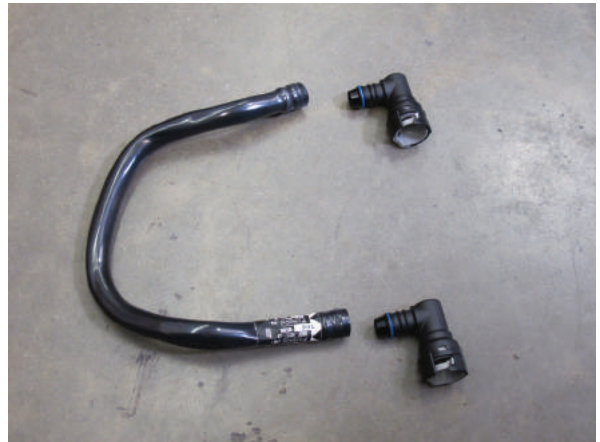
Fig. 5D-1: OEM Passenger Side PCV Hose with fittings removed
