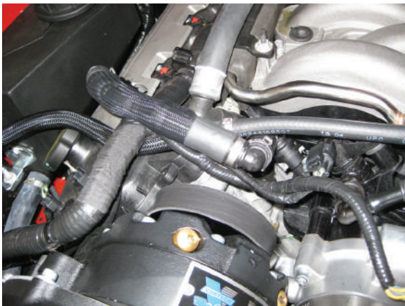
Fig. 5D-4: Modified Passenger Side PCV Hose, Installed
